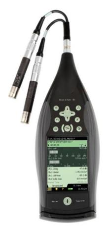
Figure 7: Example of a typical sound level meter. Retrived from the Bruel & Kjaer website on Sept. 27, 2020. https://www.bksv.com/en/products/measuring-instruments/sound-level-meter/2270-series/Type-2270-S
