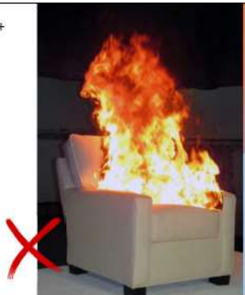
Still frames of the ISO 9705 Test Room burns for the four chair types representing flame suppression for NFR, OFFR, RFR, and BNFR at 1, 7, 11, and 14 minutes (m) from ignition.
