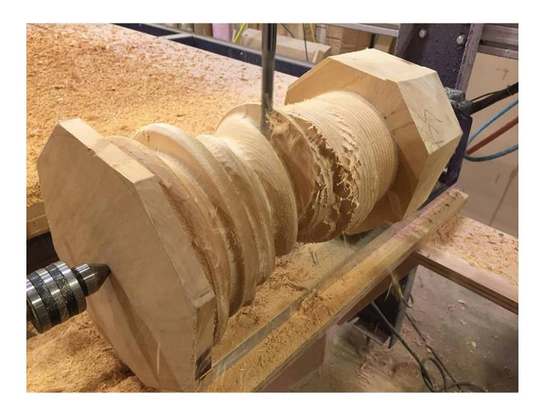
The first wood rotational milling of *Outerwear\_BW1* tears through the basswood chipping away pieces that are apart of the intended original digital design.
