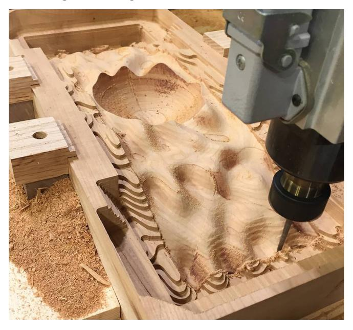
First iteration of CNC mill of *Smocked Locked*. The wall thickness of the center bowl was cut too thin during the milling, so it was placed aside.
