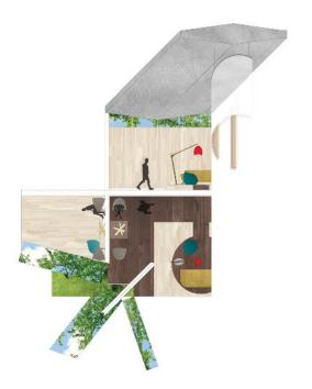
Surface > + < space: An interior elevation is a single surface alone, so students partnered elevations with floors, ceilings and adjacent walls. The unfolded drawings establish precise relationships between surface and space.
