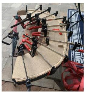
Process | Bending the wood over a particle board mold
