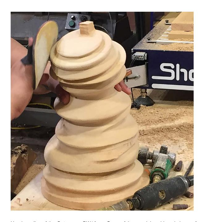
Hand sanding of the *Outerwear\_BW1* form. Some of the remaining chipped pieces of the form during the milling process can be seen here.
