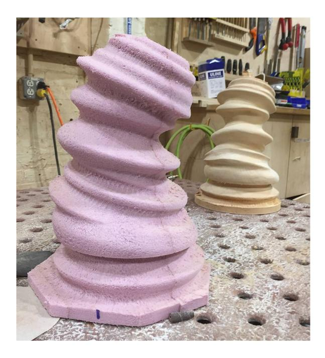
Prior to the wood milling of *Outerwear\_BW1*, a test milling was completed out of foam. The foam test was identical to the intended digital design of the work. The foam form is used as a reference for understanding the original digital file intent and to inform the hand craft process of what the potential is for the new, salvaged form.
