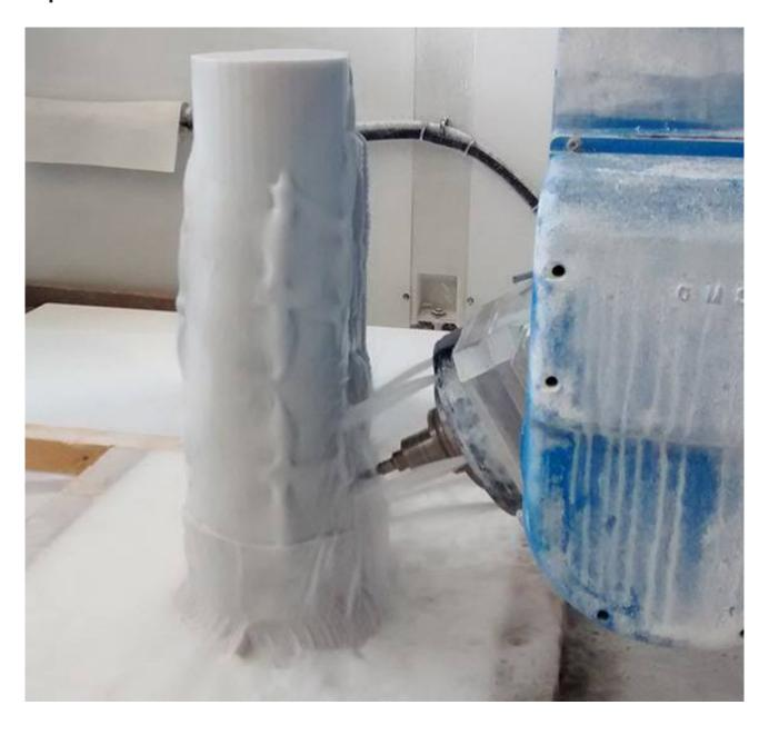
The stone work *Dug by the Devil* during the 7-axis rough milling of the sculpture. The surface exhibited some irregularity in the smoothness of the center cylinder, appearing ridged which was not the intention of the digital design.
